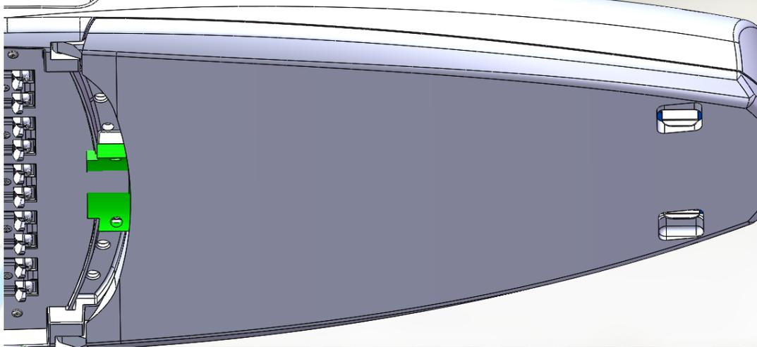
1. Loosen the four 1/2"-13 hex head bolts holding the two clamp brackets enough to slide lamp into arm approx 4.5" (125mm) deep, until arm rest on steps that would sit between the mast arm and pipe clamps and run electrical feed wires to inside of lamp terminal block.
