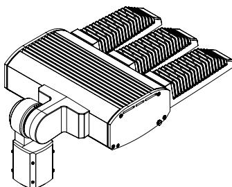
An adjustable knuckle slip fits over a 2 3/8" Tenon, and allows for up to 90° degrees of vertical adjustment in 10° degree increments from horizontal, as well as full side to side adjustment with the knuckle mount.
