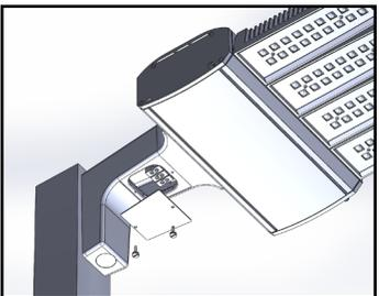
5. Remove the Access Cover Plate by unscrewing #10-24 X 3/4" Knurled Head Thumb Screws.
