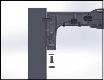
3. Secure in place with 1/2" Nord-Lock Washer and 1/2"-13 X 1-1/4" Thread Locking Hex Head Bolt. Tighten to 45 ft-lb.
