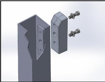
1. Align the holes in the Pole Bolster Plate, BOA Mount Casting and Pole, and secure in place with 1/2" Flat Washers and 1/2"-13 X 1-3/4" Thread Locking Hex Head Bolts. Tighten to 30 ft-lb.
